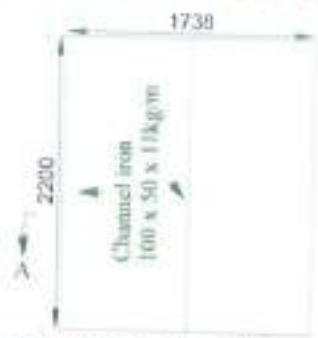
TOP VIEW: Carrier and support beams
